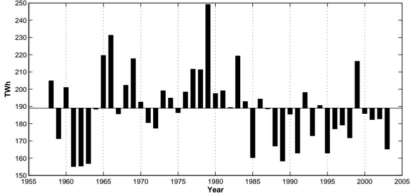
Figure 1: Water inflows, in TWh and for the period 1958–2003, to the hydropower assets of Hydro-Québec running in 2003. Displayed as surpluses and deficits against the series arithmetic average of 189 TWh.
